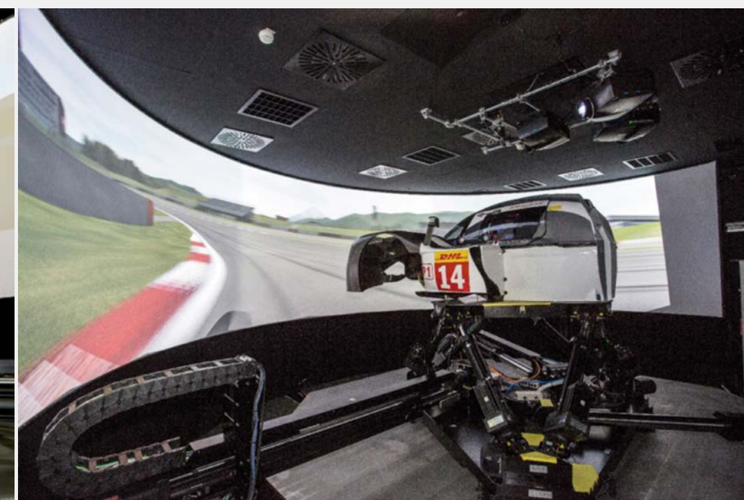
DiM – Driver-in-Motion installed at Porsche Motorsport
